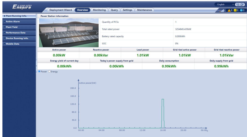
Figure 6-5 Plant running information (with power meter and battery)
