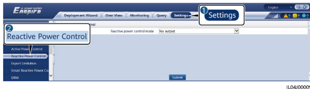
Figure 6-73 Reactive power control
