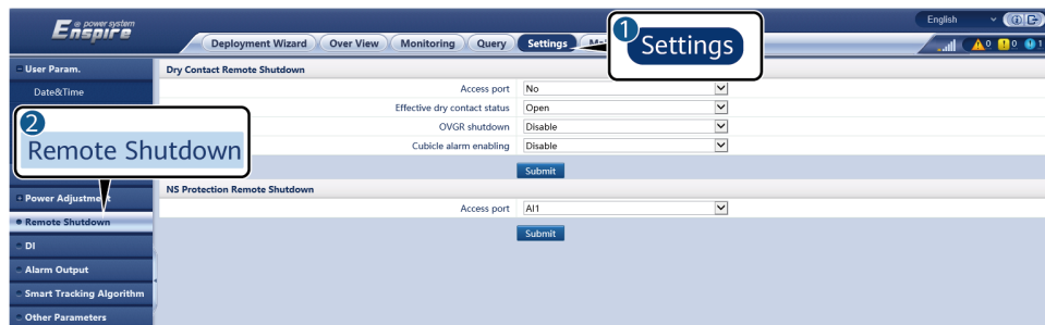
Figure 6-85 NS protection remote shutdown
