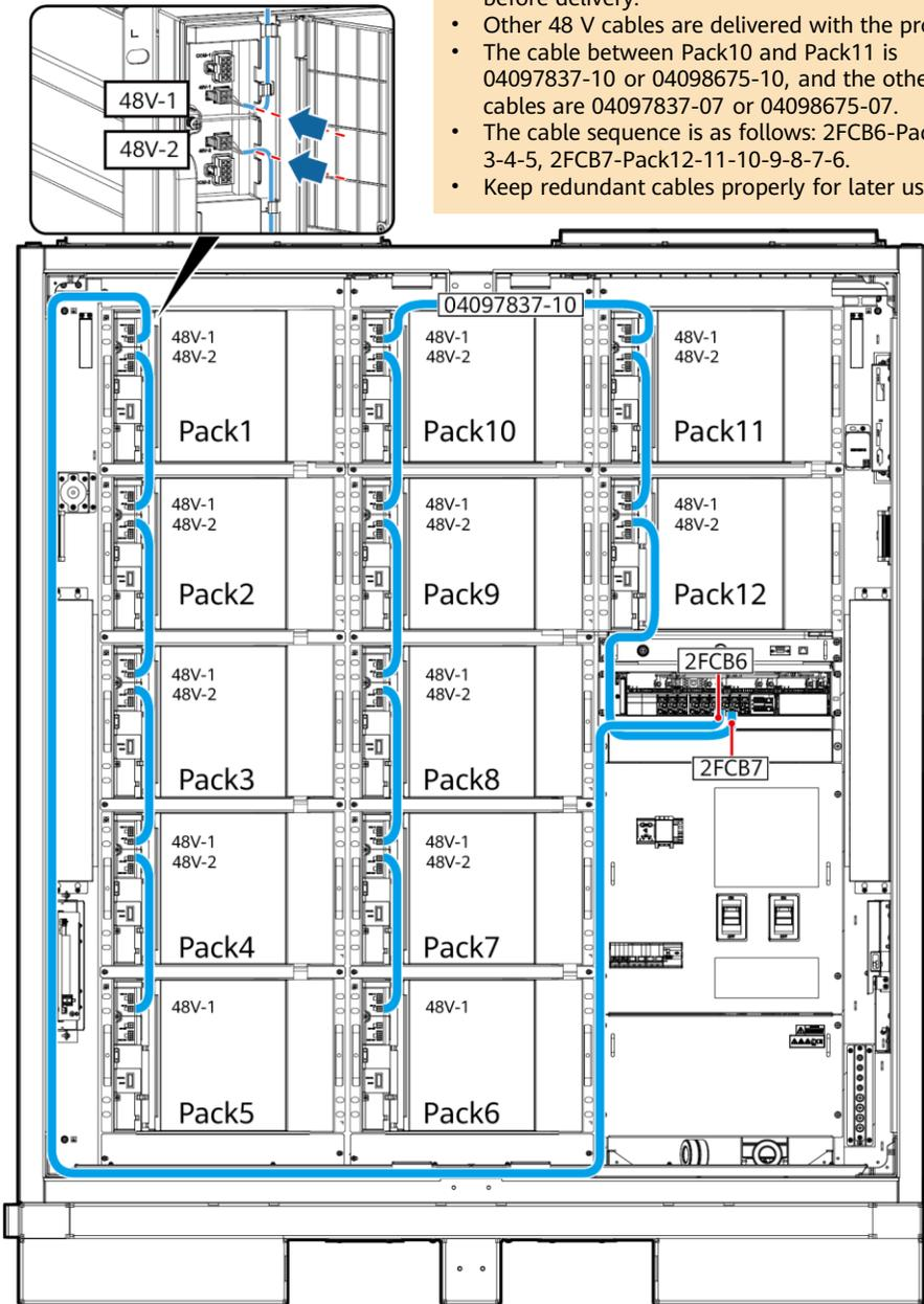
3. Install cables to the COM ports.
